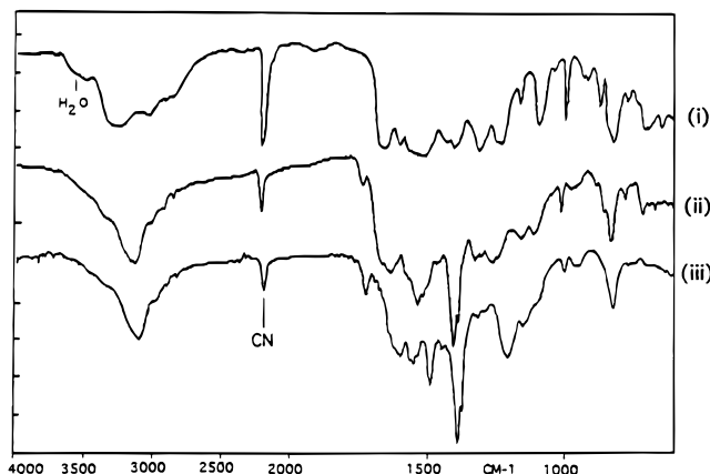
Figure 10. FTIR spectra of (i) uncured polymer 25 , (ii) polymer 25 cured isothermally in nitrogen, and (iii) poly(enaminonitrile) homopolymer cured isothermally in nitrogen.
